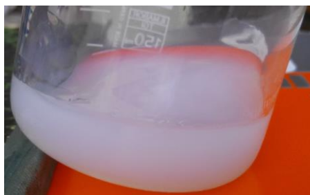
Figure 5. Nano-cellulose dispersion and nano-cellulose film obtained from TEMPO-oxidized cellulose
