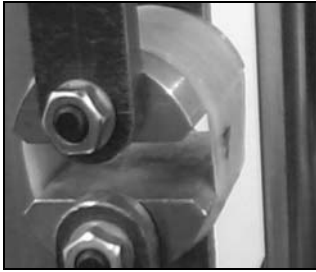
Fig. 6. Straining of rings during the testing
