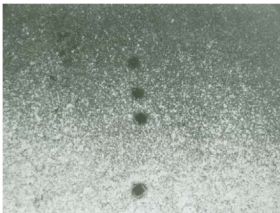
Figure 7. Fine grain ferrite-pearlite microstructure of chain bracket forging, average hardness value 220 HV. Slika 7. Finozrna feritno perlitna struktura otkovka spojnice lanca, prosečne tvrdoće 220 HV
