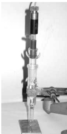
Slika 1. Fotografija male elektrohemijske ćelije za merenje korozionog potencijala čelika u kapi rastvora \text{HNO}_3 + \text{FeCl}_3 + \text{HCl} . Figure 1. Photograph of the small electrochemical cell for measuring the corrosion potential of steel in drop of the solution of \text{HNO}_3 + \text{FeCl}_3 + \text{HCl} .
