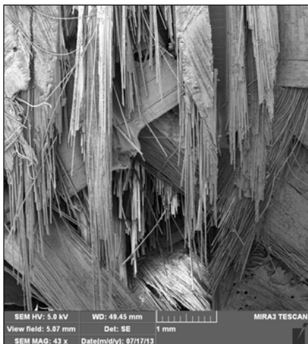
Figure 13. Different times of fiber cracking in dependence of the resin deficiency
