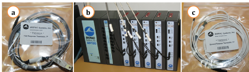
Figure 3. Physiological data monitoring system MP150 BIOPAC: MP150/100 Acquisition unit, UIM100C Universal interface module and Skin temperature amplifier modules SKT 100C (a); thermistor transducers TSD202A (b) and TSD202E (c).
