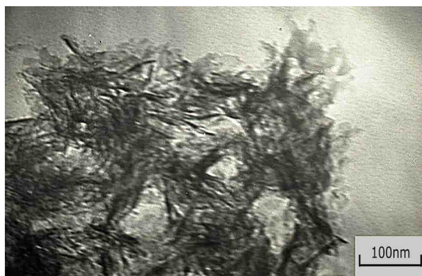
Fig. 1. Transmission electron microscopy microphotograph of hydroxyapatite/graphene (HAP/Gr) composite powder.
