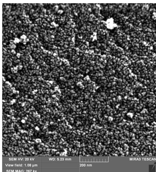
Figure 1. FESEM image of carbon cryogel/ceria composite
