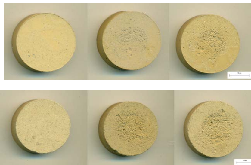
Fig.2. a) Samples without fibers before and during testing, b) Samples with 2% of fibers before and during testing.
