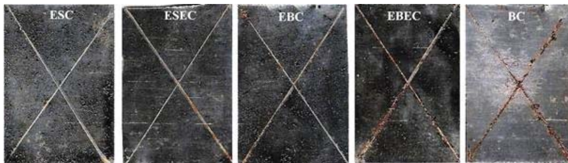
Figure 5. Comparison of the samples (4 cm x 6 cm) after treatment in a humid chamber for 5 days. Reprinted with permission of © Elsevier 2013, from ref. 24
