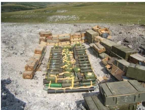
Fig. 1 Explosive devices in the pit, ready for destruction by open detonation
