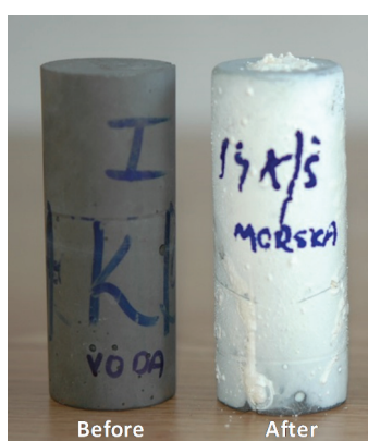
Fig. 3. Sample of AAS before and after immersion in seawater.
