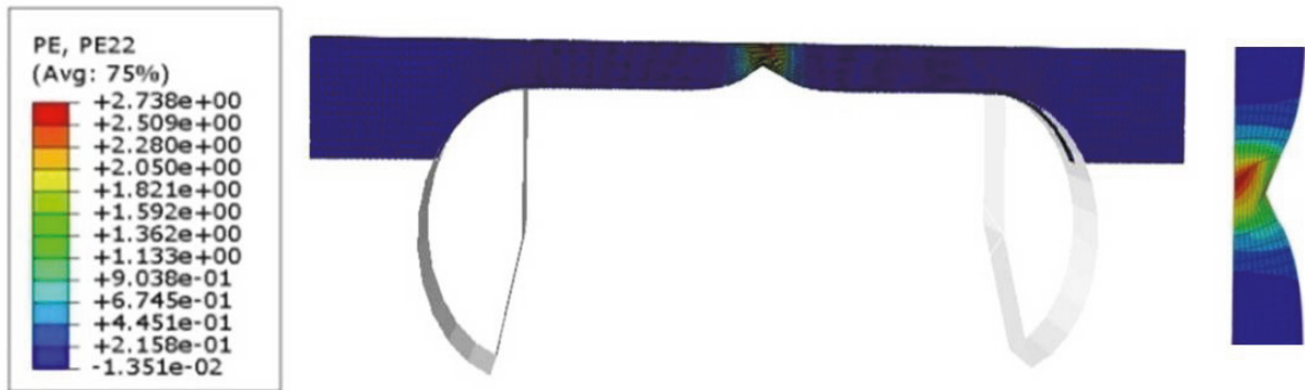
Fig. 5. The field of plastic strain of the MTS of TNZ alloy, instant before fracture.
