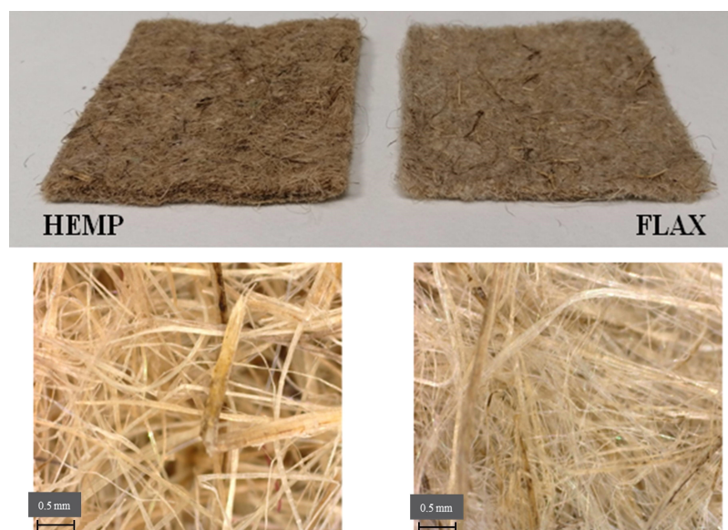
Figure 1. Hemp- and flax-based felts (below: optical microscopy images of the felt surface).
