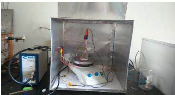
Figure 2. Faraday cage with system of electrodes
