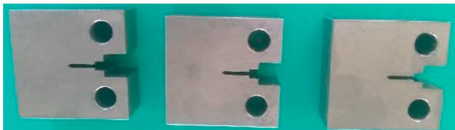
Figure 1. CT-50 specimens for fatigue crack growth rate testing at room temperature
