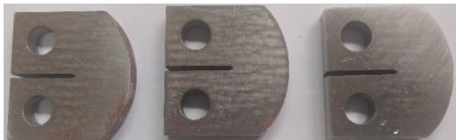
Figure 2. Modified C(T) specimens for fatigue crack growth rate testing at high temperature
