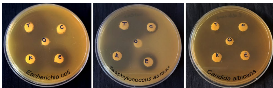
Figure 1: Antimicrobial activity of starch aerogels: neat (O) and impregnated with thymol (T), carvacrol (K), citronellol (C), and eugenol (E)
