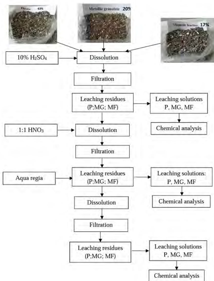
Figure 1. Technological scheme of dissolving samples for chemical analyses
