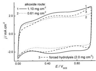
Fig. 2. Cyclic voltammograms of Ti/RuO<sub>2</sub> anodes prepared *via* the alkoxide route and the inorganic sol–gel procedure. Electrolyte: 1.0 mol dm<sup>-3</sup> H<sub>2</sub>SO<sub>4</sub>, room temperature. Sweep rate: 50 mV s<sup>-1</sup>.
