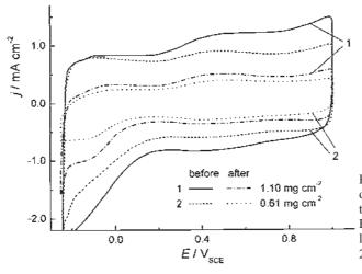
Fig. 7. Cyclic voltammograms of Ti/RuO<sub>2</sub> anodes prepared *via* the alkoxide route in 1.0 mol dm<sup>-3</sup>  $H_2SO_4$  before and after the accelerated stability test. Sweep rate 20 mV s<sup>-1</sup>.
