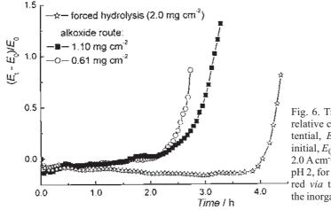
Fig. 6. Time dependence of the relative change in the anode potential,  $E_{\rm t}$ , with respect to the initial,  $E_0$ , at a current density of 2.0 A cm<sup>-2</sup> in 0.50 mol dm<sup>-3</sup> NaCl, pH 2, for Ti/RuO<sub>2</sub> anodes prepared *via* the alkoxide route and the inorganic sol–gel procedure.
