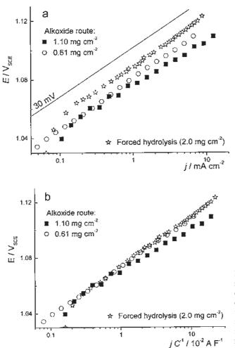
Fig. 4. Tafel plots (a) and normalized Tafel plots (b) for the chlorine evolution reaction on Ti/RuO<sub>2</sub> anodes prepared *via* the alkoxide route and the inorganic sol–gel procedure, in 5 mol dm<sup>-3</sup> NaCl, pH 2, at room temperature.
