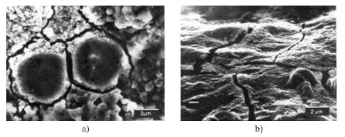
Fig. 1. SEM Microphotographs of (a) thin and (b) thick (angle of incidence: 45°) hydrous ruthenium oxide layer prepared from ruthenium ethoxide.
