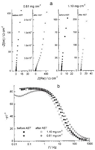
Fig. 8. Complex plane plots (a) and Bode phase angle plots (b) of the EIS data registered in 1.0 mol dm<sup>-3</sup>  $H_2SO_4$  at a potential of 0.50  $V_{SCE}$ , before and after the accelerated stability test, for Ti/RuO<sub>2</sub> anodes prepared *via* the alkoxide route.
